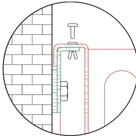
Figure 3. The analyser hanged on the holder and secured with the plastic rivets.
