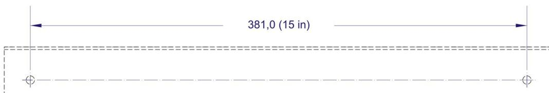
**Figure 2. Bores for the analyser without supply unit**
