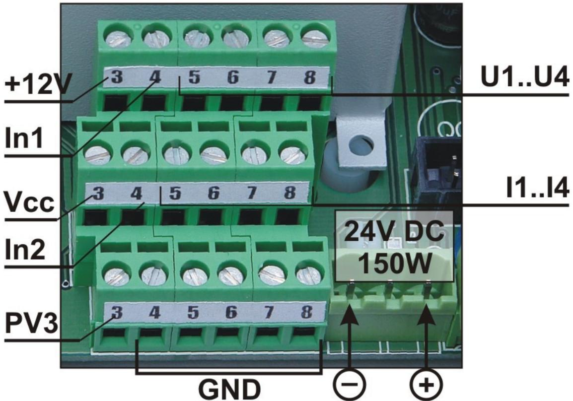
Figure 10. Power supply and the input/output connections of the *maMoS* analyser (the arrows indicate the power supply connections).
