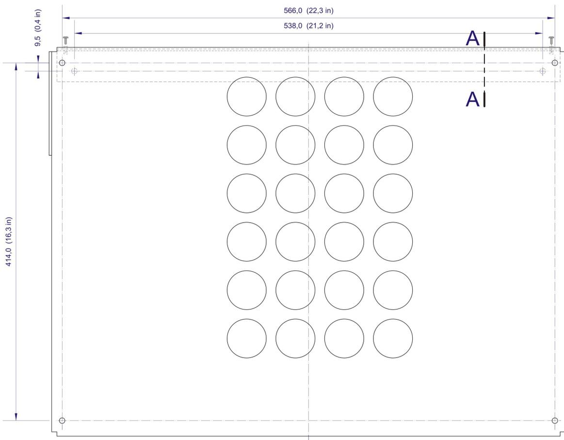
Figure 4. Location of the security holes in the analyser's holding plate (version analyser + supply)
