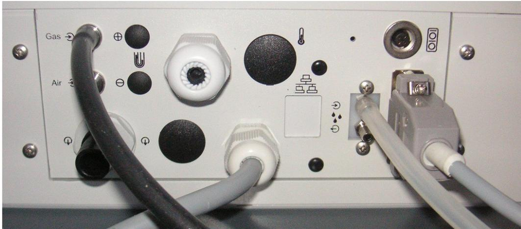
Figure 9. Electrical and gaseous connection – analyser's side
