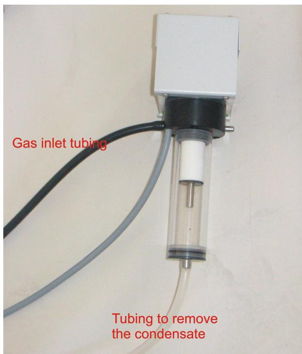
Figure 8. Gaseous connection – MD2 dryer's side
