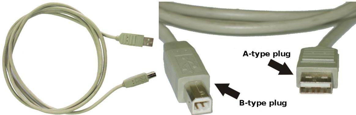
Figure 15. A connecting cable for communication via the USB interface.
