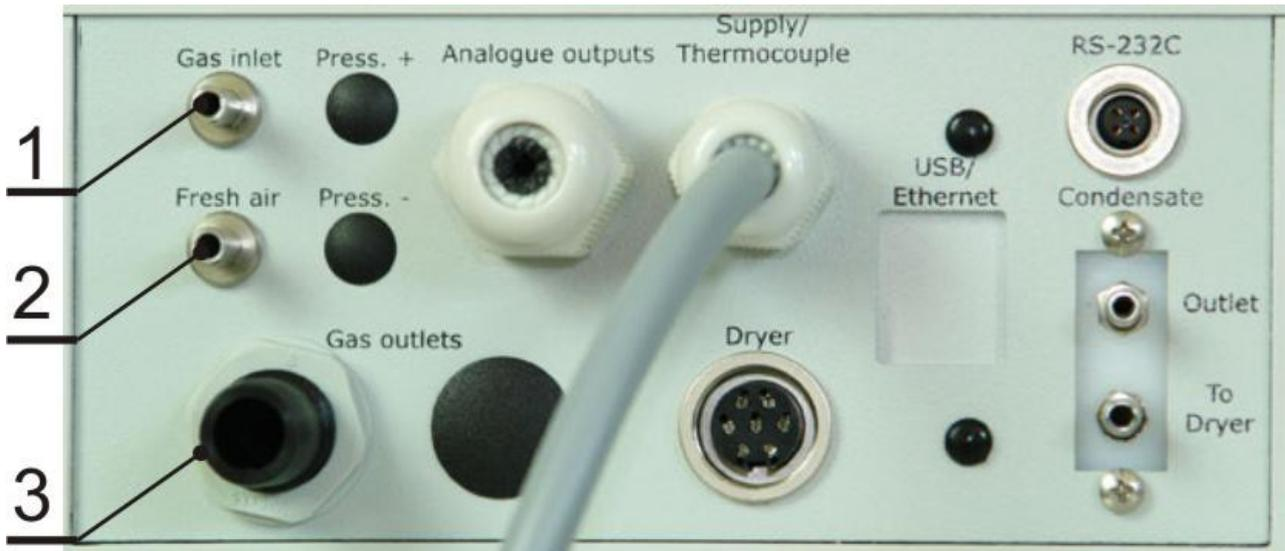
Figure 12. Connection spots (analyser with old type of dryer): 1) gas inlet hose; 2) zeroing gas inlet hose; 3) gas outlet hose.
