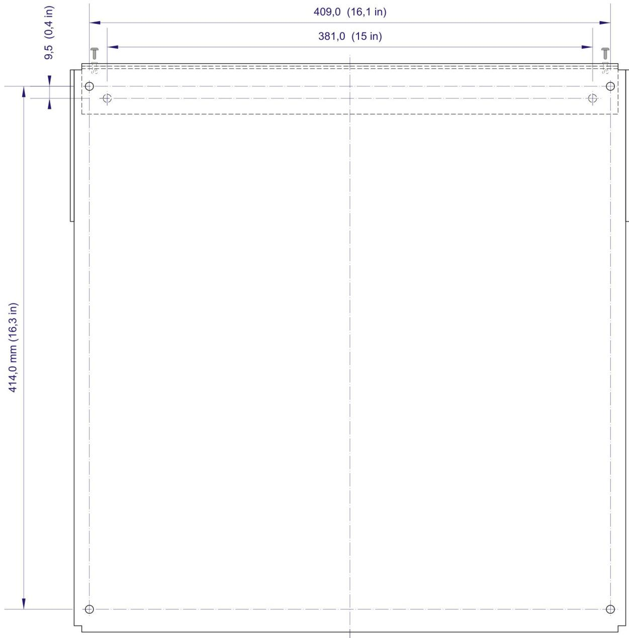
**Figure 5.** Location of the security holes in the analyser's holding plate (version analyser without supply)
